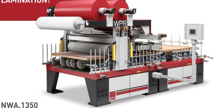
NWA 1350 is the ideal system for the lamination of nozzle application with hot melt and HMPUR adhesi-1350mm width with PVC or paper foils. This machine productivity. features all the technological advantages of slot
